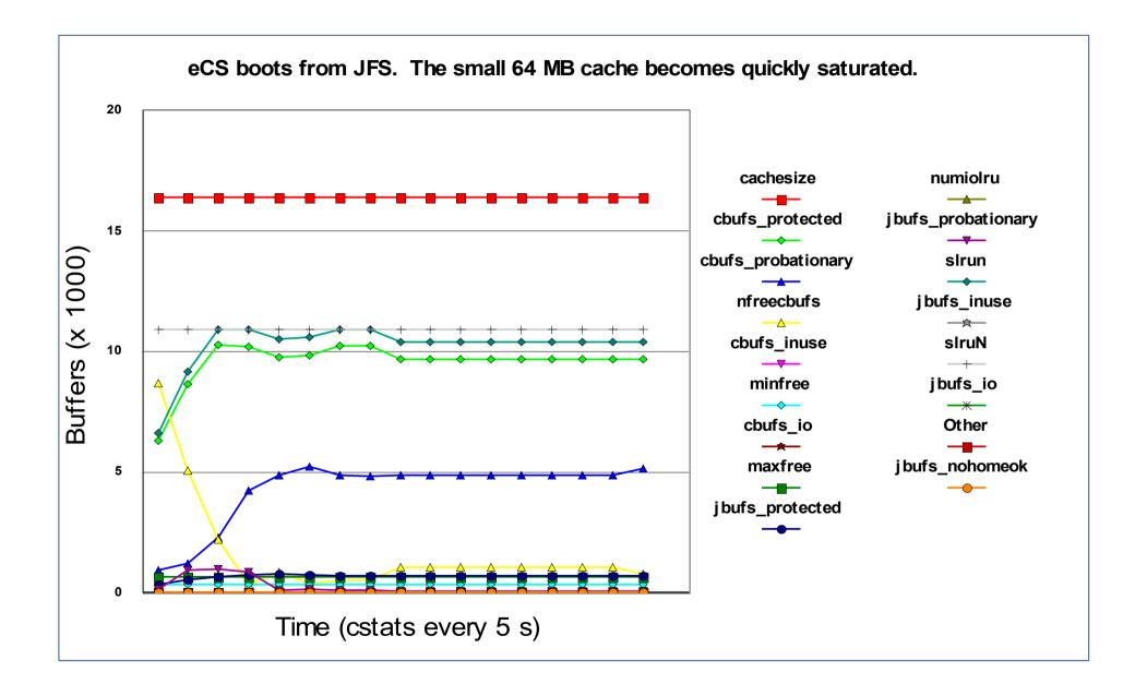
Small caches (32, 64 MiB) quickly run out of free buffers, but are also more easy to synchronize (less stuff to be cached).
